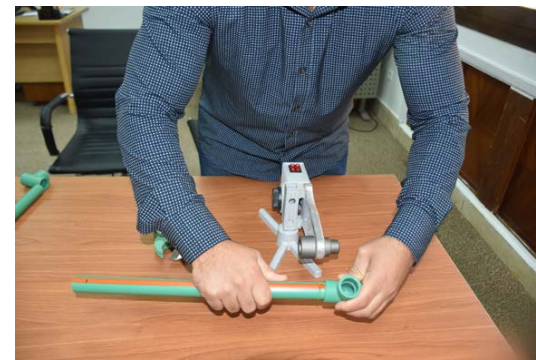
4. At the end of heating period fitting and pipe end from the heating elements have to be pulled off fully and simultaneously.
