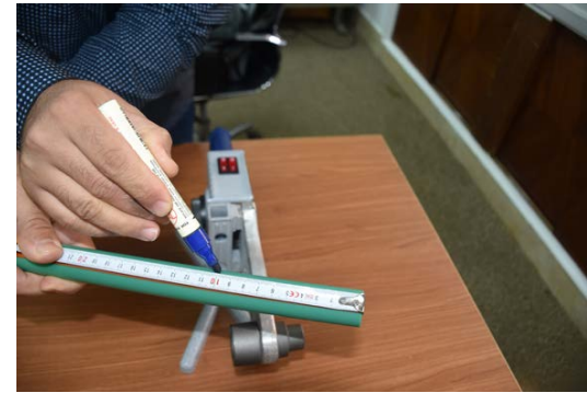
2. Clean the joint area with cleaner. Mark the insert depth of the fitting on the pipe.
