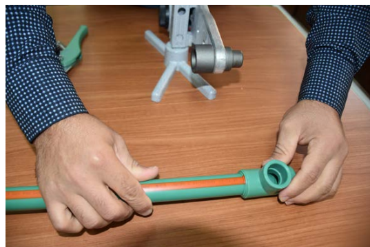
5. Adapt and join pipe and fitting within the max. allowed period without turning the parts against each other.
